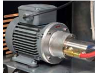
Gear Pump for refrigerant charging.
