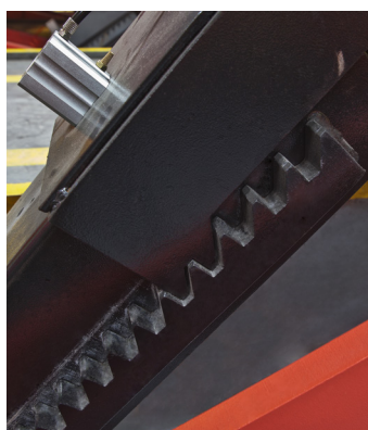
15 Level Locking Positions with Pneumatic Lock Release System
